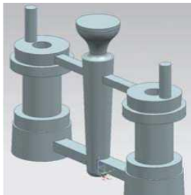
Figure 1 – 3D model of the gating-feeding system
