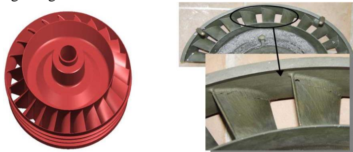
Figure 1 – Cracks that occur during the casting of gas turbine engine blades due to high stresses in the casting
